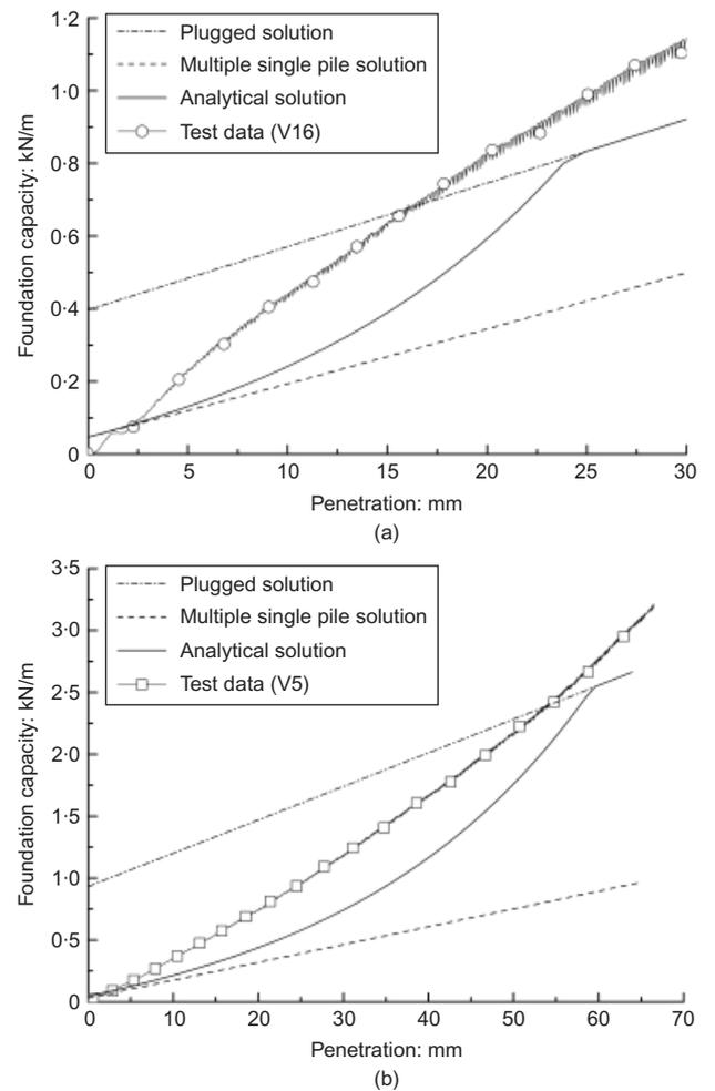
Fig. 5. Comparison of analytical solutions with load test data: (a)  $s/t = 2.5$ ; (b)  $s/t = 4$  ( $\phi = 30.8^\circ$ ;  $\delta = 21.7^\circ$ ;  $\gamma = 14.59 \text{ kN/m}^3$ ;  $K = 1.5K_0$ )
