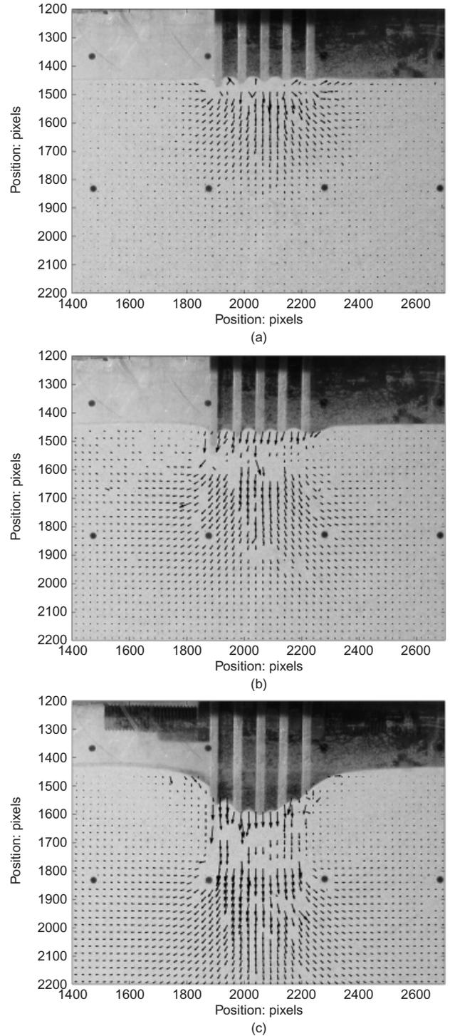
Fig. 12. Incremental soil displacements observed in test V16 ( $s/t=2.5$ ): (a) increment  $z=0-6$  mm; (b) increment  $z=18-24$  mm (onset of plugging); (c) increment  $z=47-53$  mm (maximum allowable penetration)
