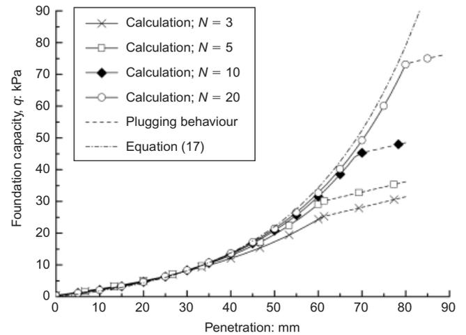
Fig. 9. Calculation of foundation capacity–penetration relationship (loose sand;  $s/t = 4$ ;  $t = 5$  mm)
