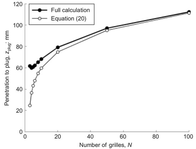
Fig. 10. Calculated plugging penetration against number of grilles (loose sand;  $s/t = 4$ )
