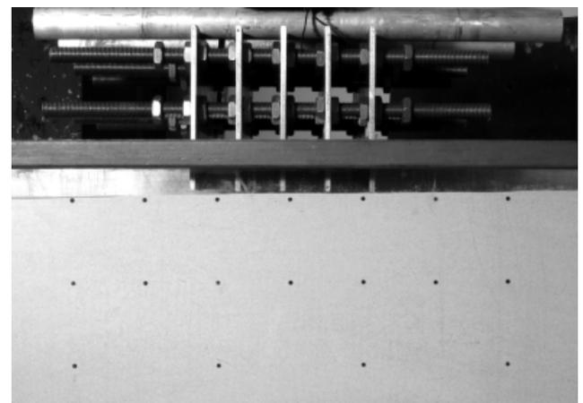
Fig. 3. Vertical grillage testing apparatus: (a) schematic diagram of apparatus; (b) photograph of grillage foundation ( $N = 5$ ,  $t = 5$  mm,  $s/t = 8$ )
