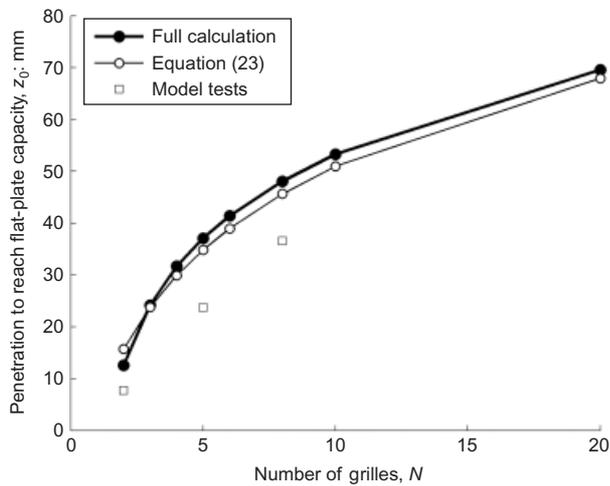
Fig. 15. Calculated penetration to reach flat-plate capacity ( $s/t = 4$ ; loose sand)
