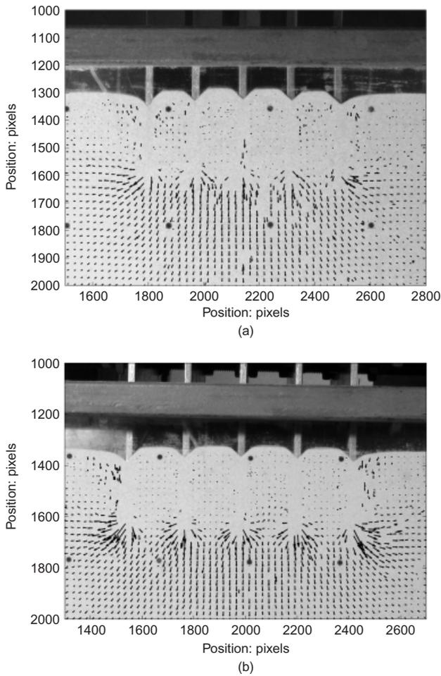
**Fig. 13. Observed incremental soil displacements at full penetration of grillage ( $z \approx 50$  mm): (a) test V18 ( $s/t = 6$ ), increment  $z = 47\text{--}53$  mm; (b) test V11 ( $s/t = 8$ ), increment  $z = 49\text{--}55$  mm**
