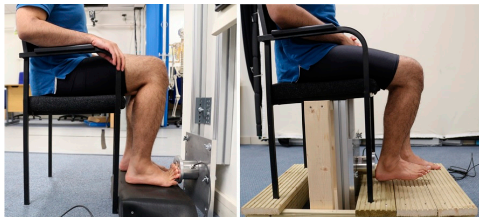
Figure 4. Measurement of the toe- or heel-forces when participants sat with the knee extension (left) or knee flexion (right).
