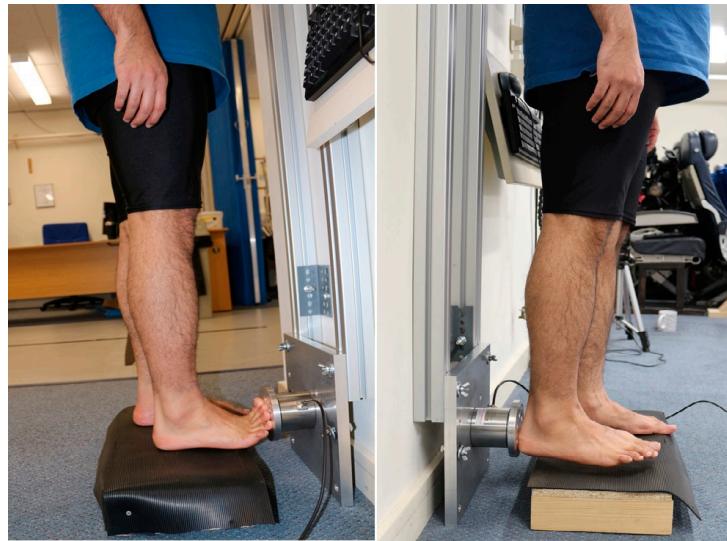
Figure 3. Measurement of toe- or heel-forces when participants stood and performed hip flexion (left) or extension (right).
