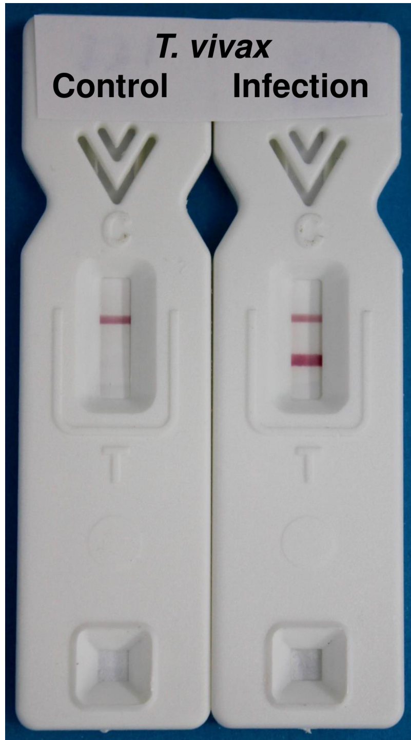
Fig 2. Examples of the TvY486_0045500 prototype lateral flow tests developed with control and infection sera, as indicated. Top band control line, bottom band TvY486_0045500 diagnostic line.
