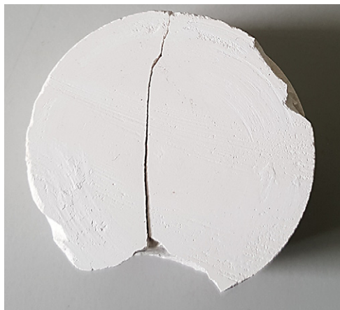
Figure 6. Tensile failure of a dry chalk sample sheared at 1000 kPa
