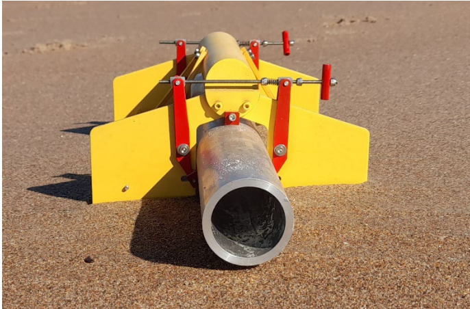
Figure 16 VEPLA concept model shown clamped to a pipeline mock-up
