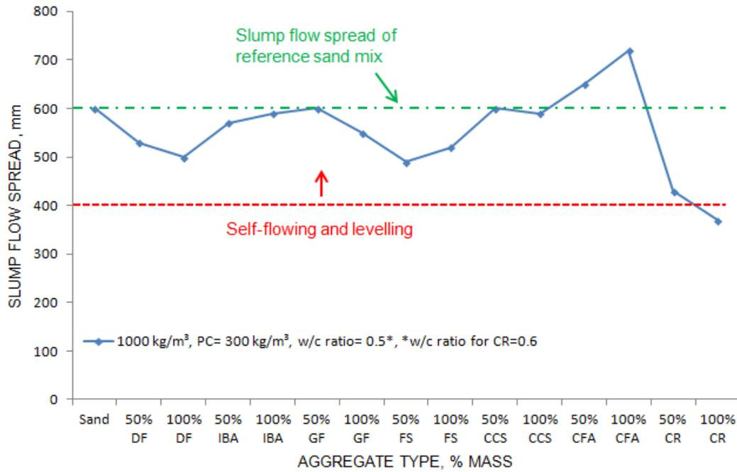
Figure 2 Relationship between aggregate type and slump flow [6]
