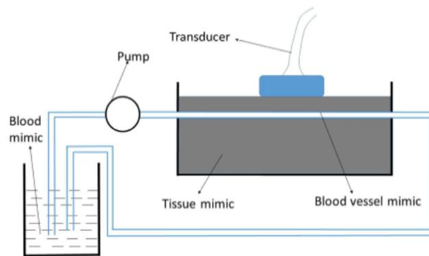
Figure 1. The diagram of the flow phantom
