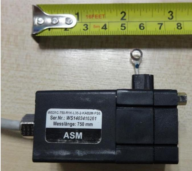
Figure 3. Draw-wire potentiometer WS31C.
