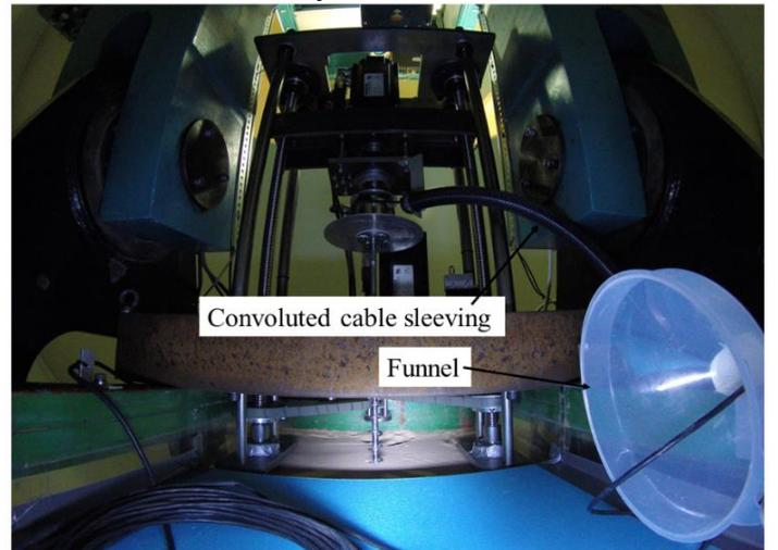
Figure 5. Screw pile installation in flight at 50-g.
