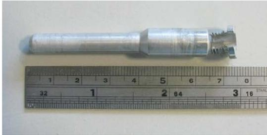
Figure 8. The mid height pore pressure transducer attachment used for 180,000% repeat test.
