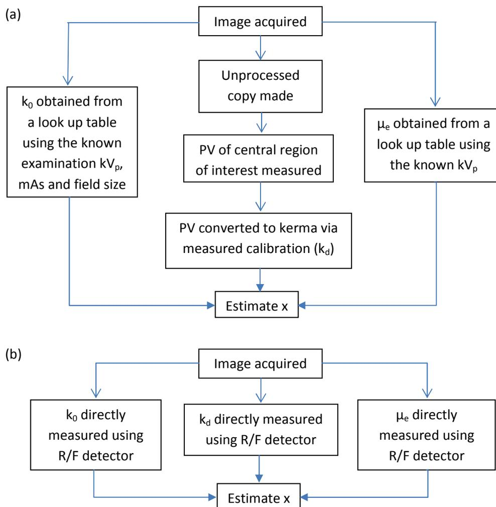
Figure 6: Estimating attenuator thickness using (a) estimates of  $k_d$ ,  $k_0$  and  $\mu_e$  made using the model presented in this paper and (b) direct measurements of  $k_d$ ,  $k_0$  and  $\mu_e$
