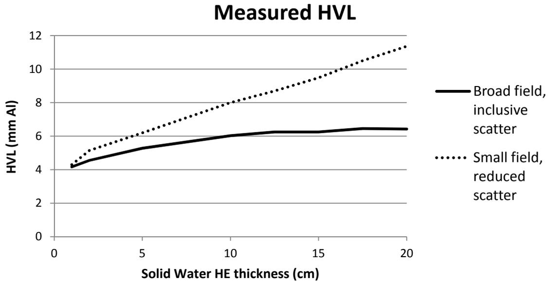
Figure 2: The broad and narrow field HVLs measured for increasing thicknesses of attenuator at 81kV<sub>p</sub>
