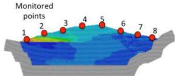
Figure 3 Monitoring points for velocity in stability analysis and velocity contours at failure.
