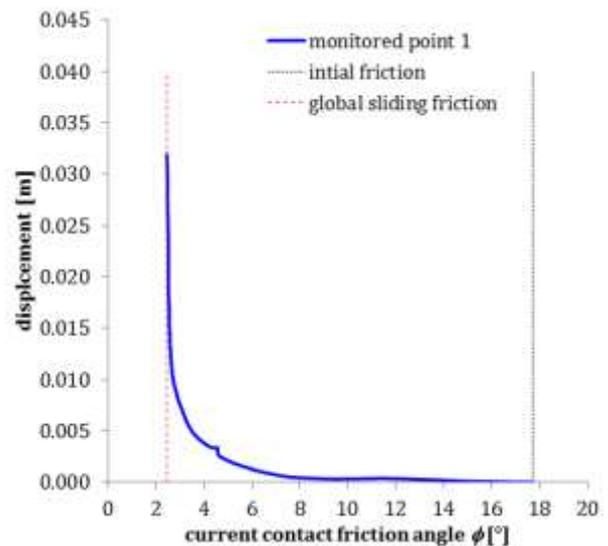
Figure 4. Displacement history at monitoring point
