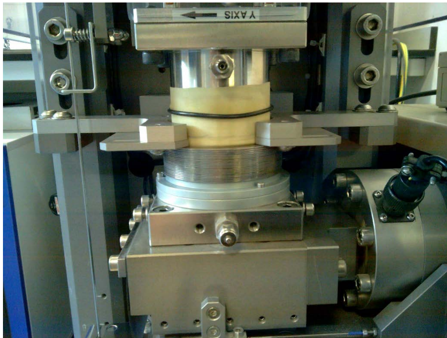
Figure 6. A50 silica sample preparation for simple shearing testing
