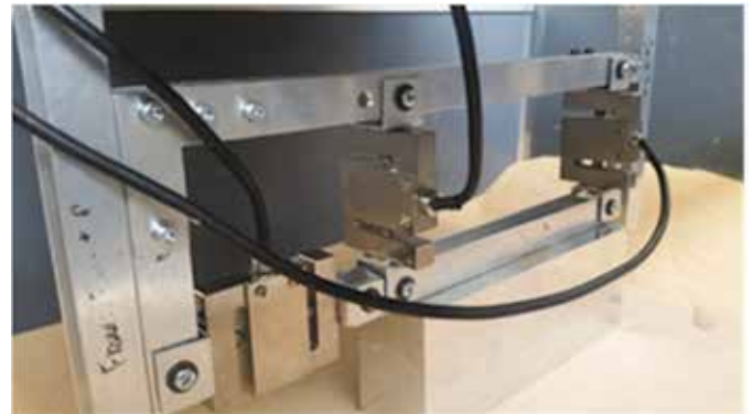
Figure 4: Load measurement frame
