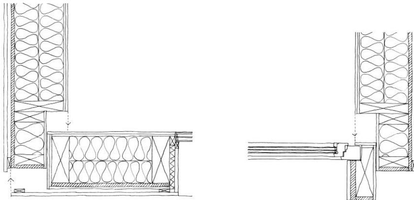
Figure 7. Passive-Energy housing in Dornbirn: horizontal sections showing assembly joints between panels.
