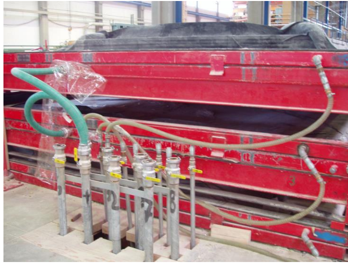
Figure 1. Manufacturing of cross-laminated timber panels: vacuum press.
