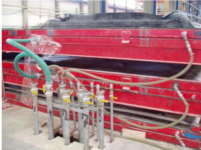
Figure 1. Manufacturing of cross-laminated timber panels: vacuum press.
