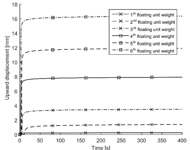
Fig. 4 upward pipe displacement at different unit weight ( $w=214\%$ ). The "1<sup>st</sup> floating unit weight" represent the heaviest pipe unit weight, the "6<sup>th</sup> floating unit weight" represent the lightest pipe unit weight. (Unit weights have been omitted for confidentiality reasons)
