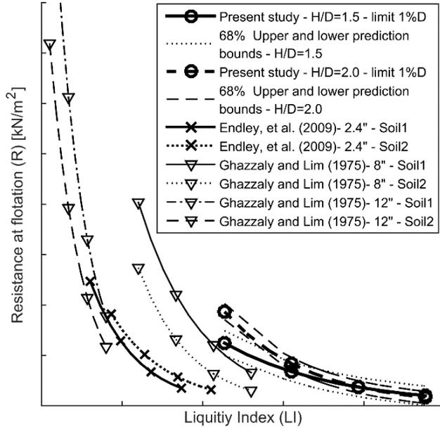
Fig. 7 Flotation criterion interpolation comparison from Ghazzaly and Lim (1975) and Endley, et al. (2009) and first fit of the present study interpolated data to the previous studies at  $1.0\%D$  displacement. (Values have been omitted for confidentiality reasons)
