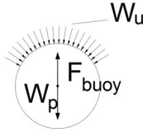
Fig. 1 Flotation equilibrium representation  $W_p$ =weight of the pipe/cable per unit length,  $F_{buoy}$ =buoyancy force per unit length,  $W_u$ =resistance provided by the mobilized soil mechanism per unit length.
