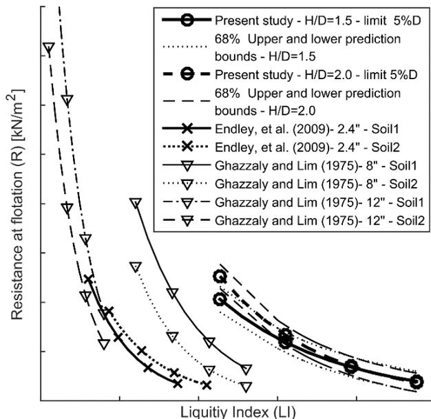
Fig. 8 Flotation criterion interpolation comparison from Ghazzaly and Lim (1975) and Endley, et al. (2009) and first fit of the present study interpolated data to the previous studies at  $5.0\%D$  displacement. (Values have been omitted for confidentiality reasons)
