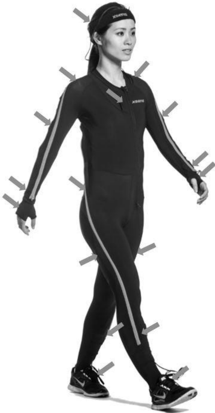
Figure 2 – Standardised placements of inertial sensors as prescribed by XSens Technologies B.V. (with kind permission from Xsens Technologies B.V.)
