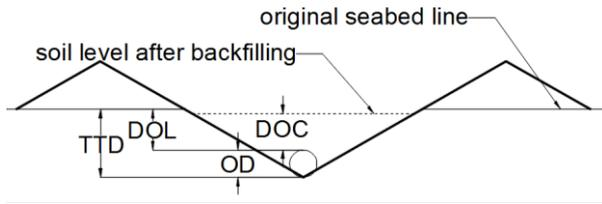
Figure 1. 2D schematic representation of a section of a post-lay ploughed trench, where TTD is target trench depth, DOL is depth of lowering, OD is the pipeline outer diameter and DOC is depth of cover after backfilling.
