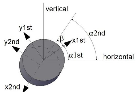
Figure 6. accelerometer axis representation. 1<sup>st</sup> represents the axis of the accelerometer near the front Perspex window and the 2<sup>nd</sup> is the accelerometer near the back wall.  $\beta$  is the out of phase angle between the two x axes of the front and back accelerometers.
