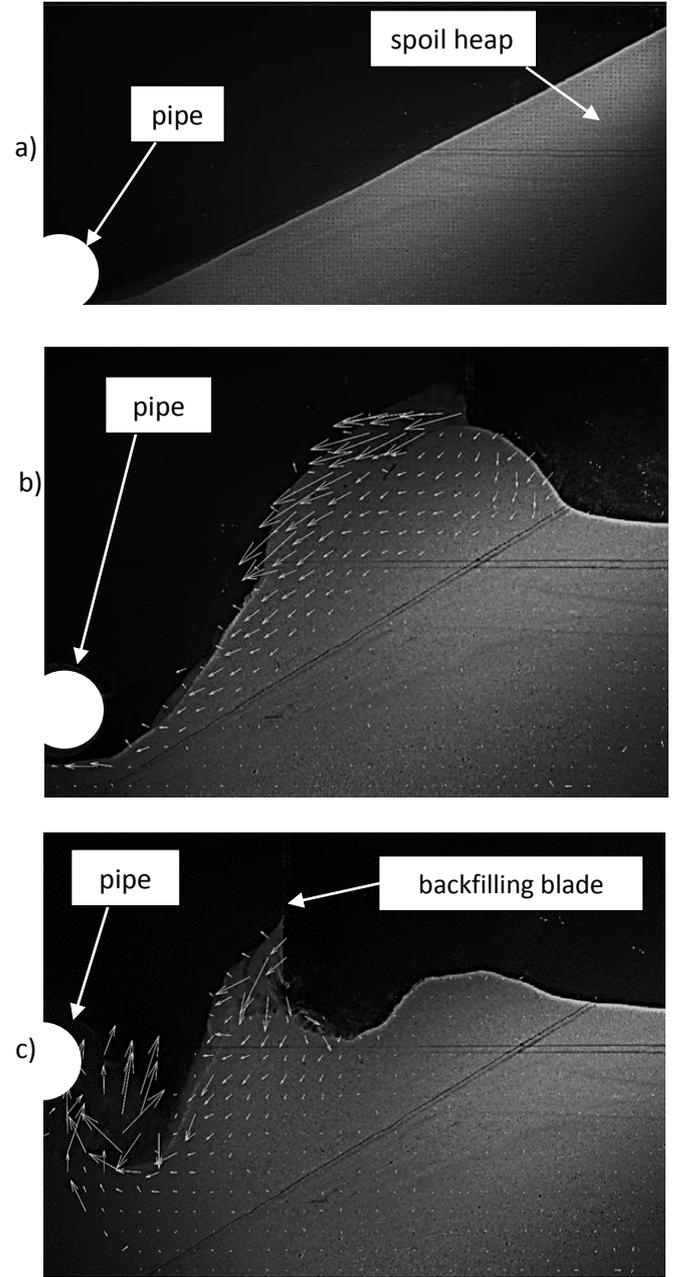
Figure 11. PIV results superimposed on the original images of a test with the large-scale model. The sequence shows the displaced pipe. a)  $t = 0$  s: initial frame for reference; b)  $t = 6.7$  s: the spoil heap is completely mobilized and the flow is starting to move downward; c)  $t = 9.8$  s: the soil flow has impacted on the pipe and is dragging it upward. The soil used for the tests is a HST95 sand as in Lauder, et al. (2013).
