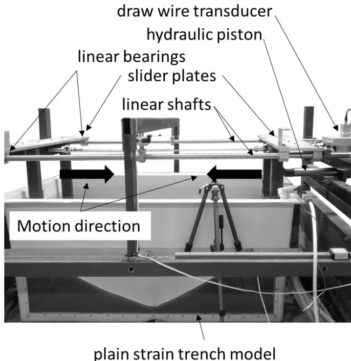
Figure 5. Model 1:7.5 2D backfilling rig actuation system.
