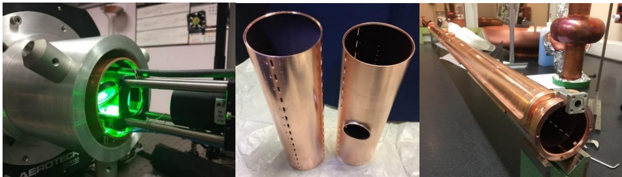
Figure 1. Manufacturing phases (left to right): LESS treatment, lateral and central treated segments, final assembled BS.
