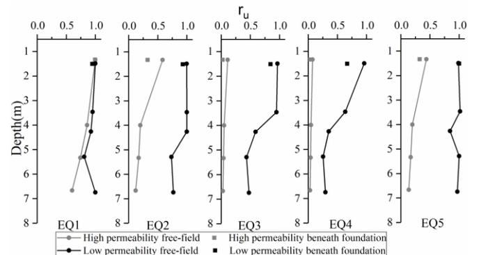
Figure 4 Excess pore pressure ratio ( $r_u$ ) along depth
