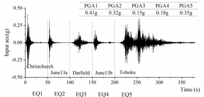
Figure 3 Input acceleration time history and peak ground acceleration (PGA)
