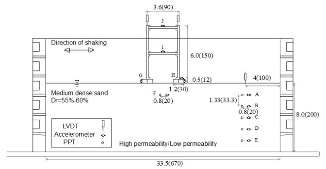
Figure 2 Layout of centrifuge test: dimensions in prototype are shown in m; dimensions in model scale are shown in mm in brackets ( ).
