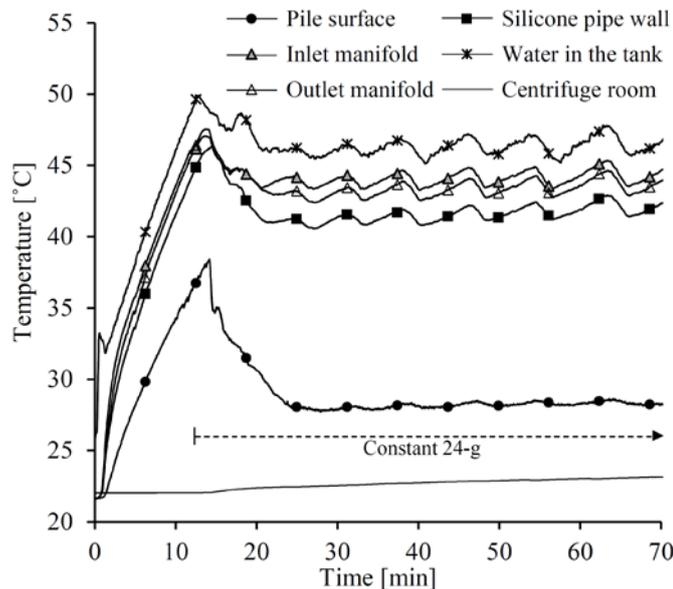
Figure 4. Temperature recorded during Test 2. Both the heating element and the pump were switched on at  $t=0$  min. The spinning was started at  $t=2$  min. Thermocouple positions are shown in Figure 1.
