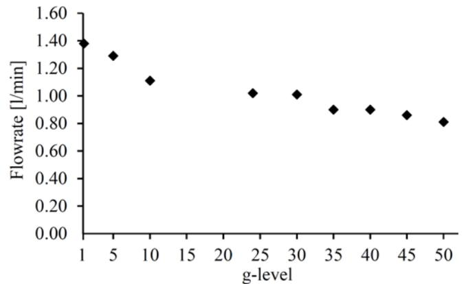
Figure 3. Steady-state flowrate (model scale) at different g-levels.
