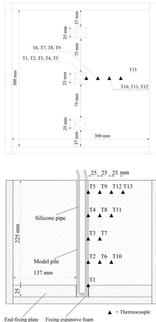
Figure 5. Plan view (top) and elevation view (bottom) of the centrifuge test setup in Test 4. Note that only results from T2, T4, T8 and T11 are presented in this paper.
