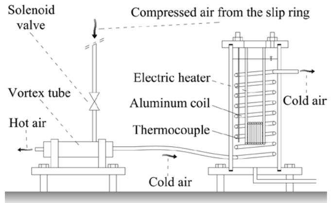
Figure 7. Schematic of the proposed cooling system.
