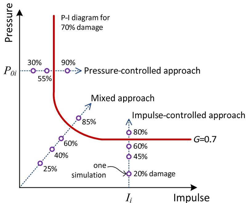
Fig. 2. Numerical derivation of P-I diagrams
