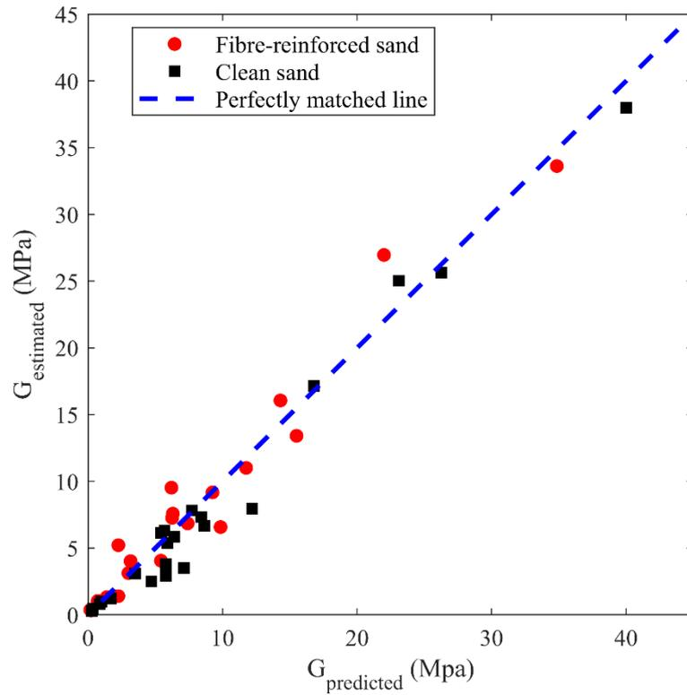
Fig. 12 Comparison between estimated and predicted shear moduli
