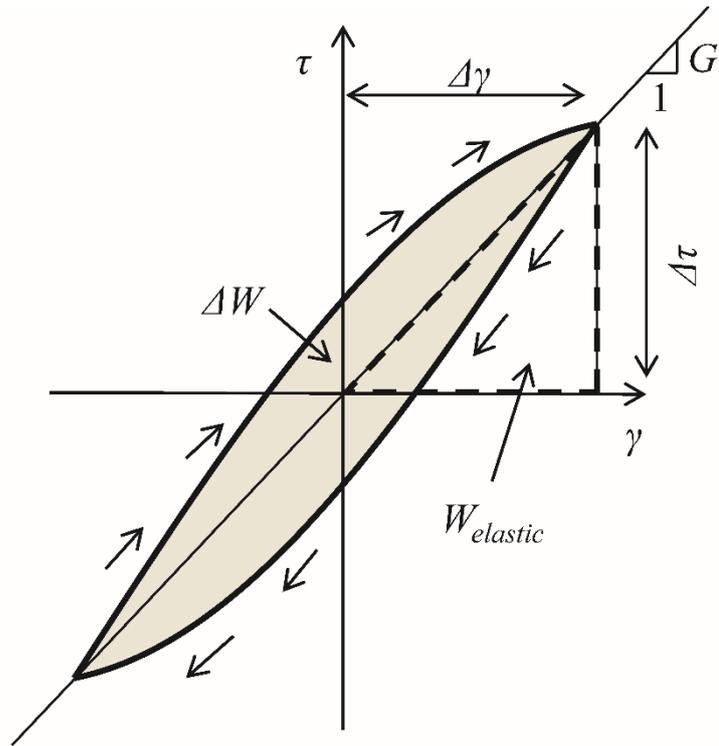
Fig. 8 Schematic demonstration of a shear stress-strain relationship
