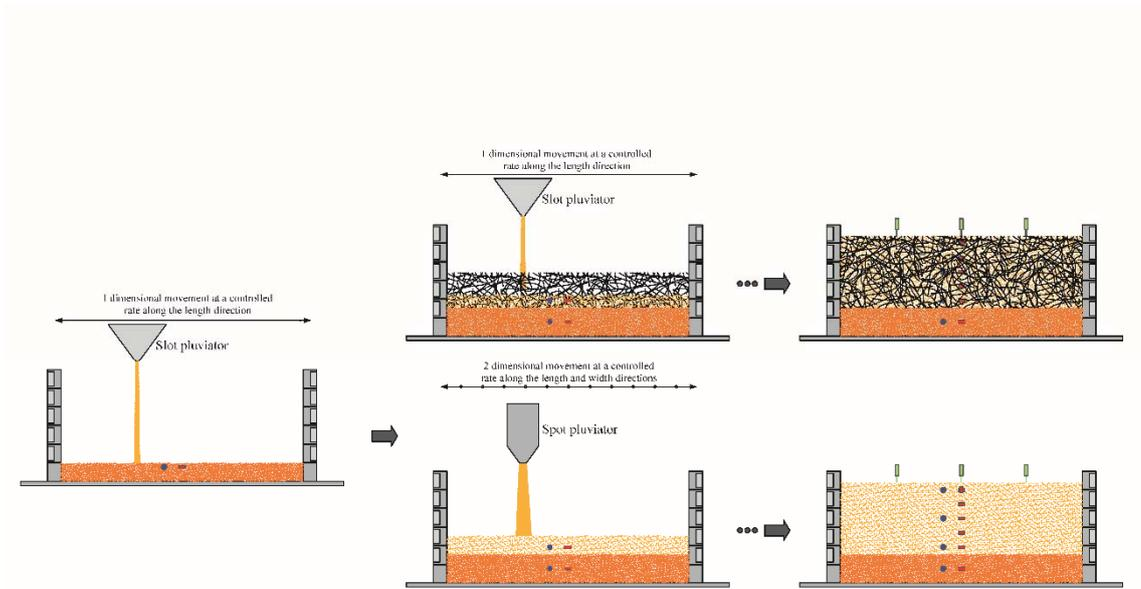
Fig. 3. Dry pluviation procedures
