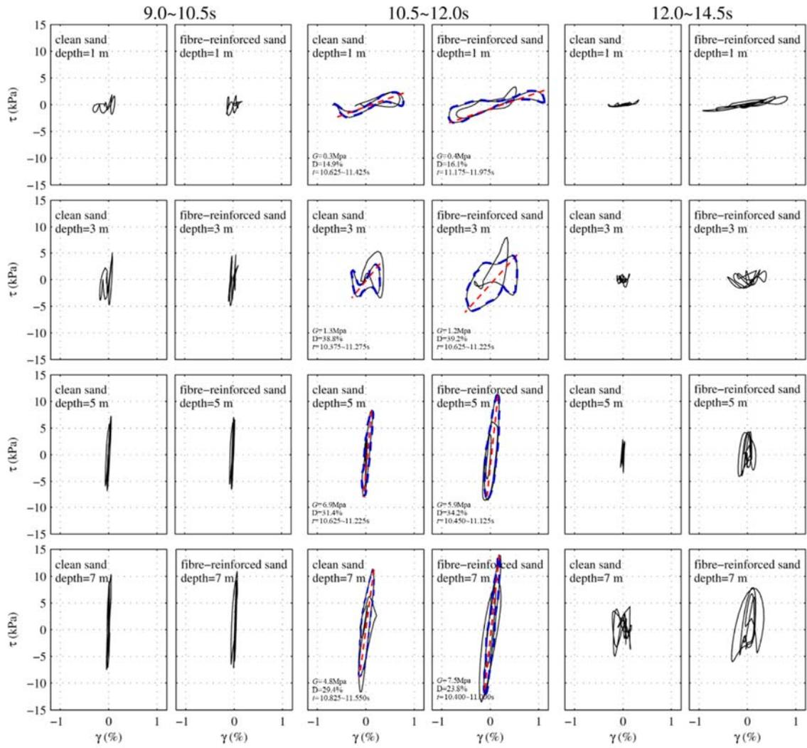
Fig. 9 Shear stress strain time histories at various depths
