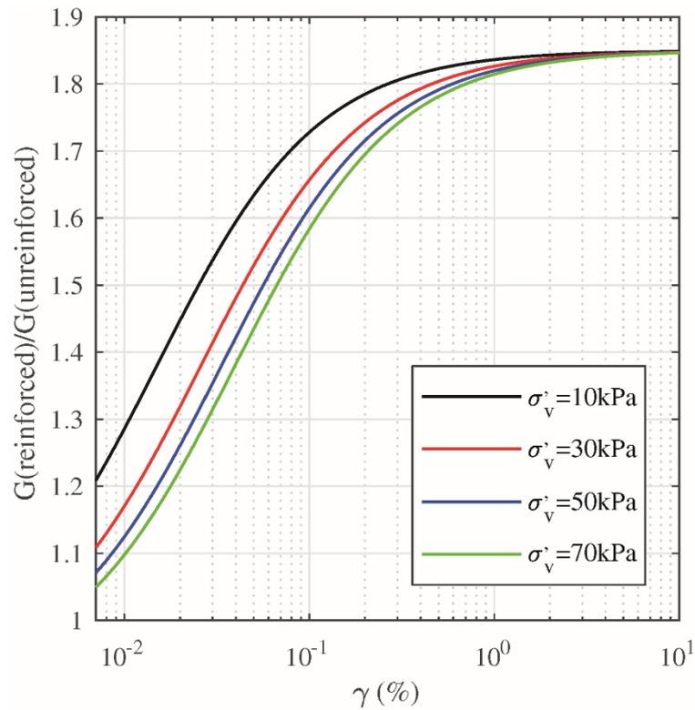
Fig. 13 Influences of  $\gamma$  and  $\sigma'_v$  on the contribution of fibres to shear modulus
