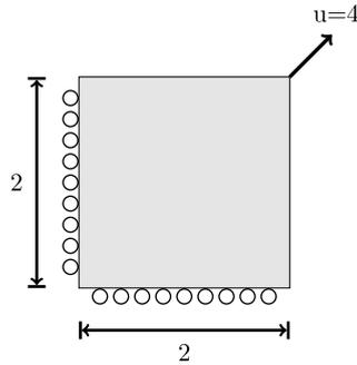
Fig. 14. Corner stretch: the geometry and boundary conditions. Left and bottom are constrained with a roller boundary condition, and the top-right corner is stretched by a total displacement boundary condition  $u = 4$  in both directions.
