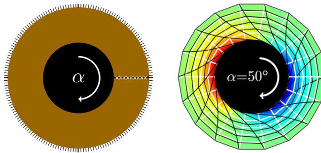
**Fig. 19.** Circular annulus: geometry with boundary conditions and FE mesh for the annulus. The outside is fixed and inner surface is rotated. The white cross markers indicate the position for sampling displacement. The white and black lines show the initial and deformed meshes in the finite element analysis, respectively.
