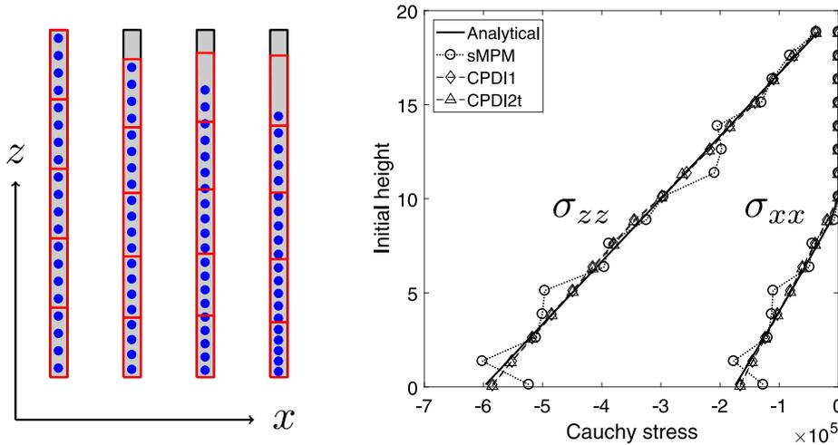
**Fig. 3.** Column compression: initial and deformed meshes with incremental deformation (red) including material points (blue). The stress components along the initial height are shown for the mesh with 20 elements with 4 material points per element. (For interpretation of the references to colour, the reader is referred to the web version of this article.)
