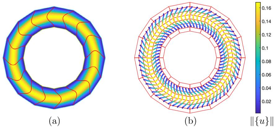
**Fig. 9.** Manufactured torsional deformation: the analytical (a) and numerical (b) deformation field with the coarse mesh ( $rf = 1$ ). The colour shows the magnitude of displacement. (Please refer to the coloured version online.)
