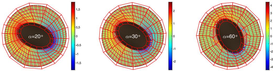
**Fig. 23.** Elliptical annulus: incremental mesh deformation at the end of the load step for  $\alpha = 20^\circ$ ,  $30^\circ$  and  $60^\circ$ , with the coloured material points showing the total vertical displacement in the sMPM simulation.
