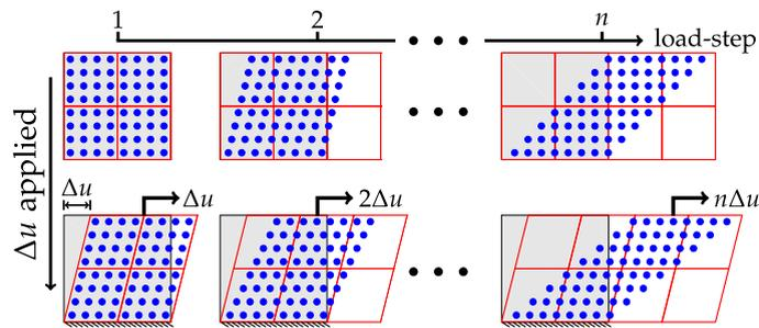
**Fig. 1.** Demonstration of the standard MPM under simple shear: a high quality mesh (red) is used in the computation of equilibrium for each loading increment, while the material points (blue) track the total deformation. (For interpretation of the references to colour, the reader is referred to the web version of this article.)
