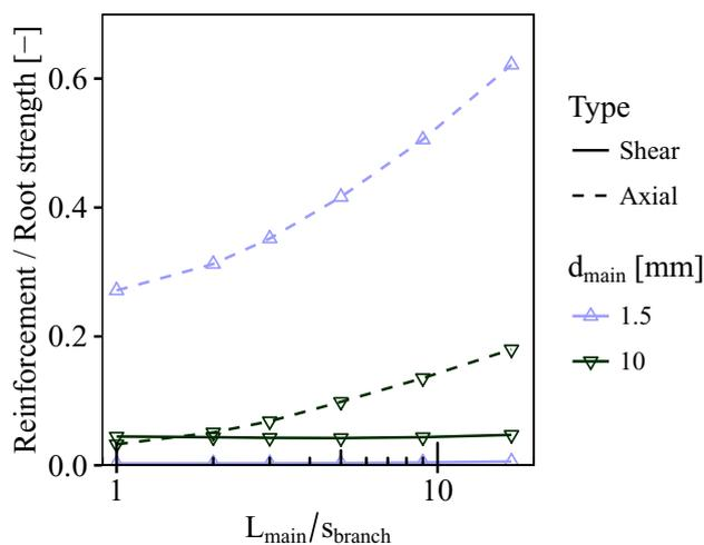
**Fig. 4.** Contributions of internal root normal and shear forces towards root-reinforcement as function of branching distance, at a shear displacement of 20 mm. Reinforcements are normalised by the maximum tensile strength of the root.
