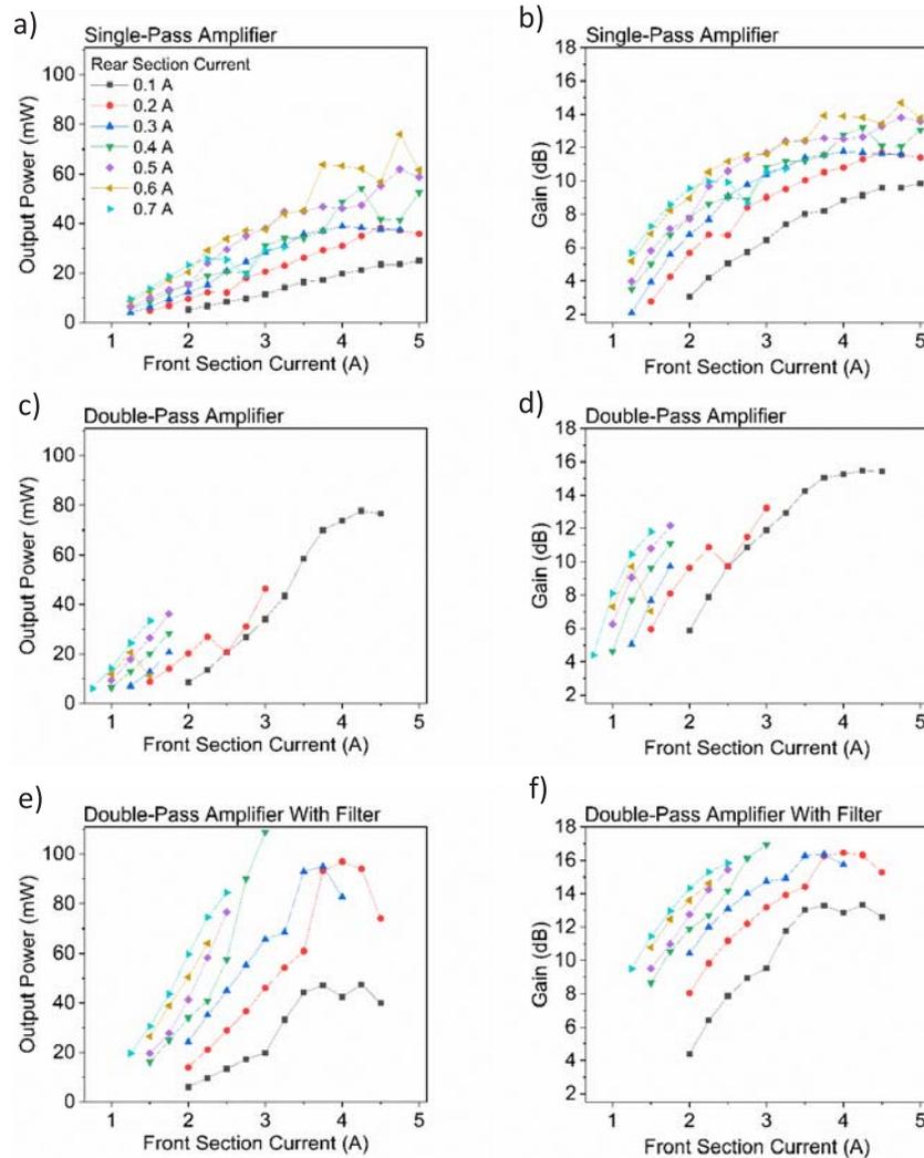
**Fig. 4.** Plots of average power and gain vs front section current at various fixed rear section currents and a constant input power around 2 mW. (a) Single-pass output power. (b) Single-pass gain. (c) Double-pass output power. (d) Double-pass gain. (e) Double-pass output power with long-pass filter. (f) Double-pass gain with long-pass filter.
