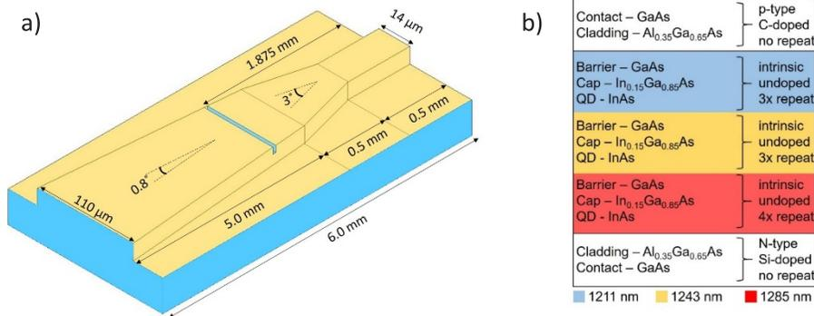
**Fig. 1.** (a) Schematic diagram of the tapered SOA, fabricated by III-V Lab (not to scale, waveguide tilt not shown). (b) Schematic illustration of the epitaxial structure used to fabricate the tapered SOA (grown by Innolume GmbH).
