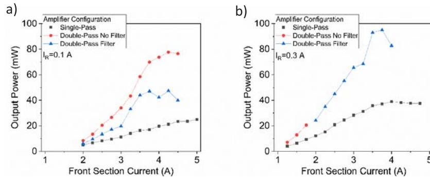
**Fig. 5.** Comparison of the output power vs front section current plots from the single-pass and double-pass configurations with and without the long-pass filter at rear section currents of 0.1 A (a) and 0.3 A (b).
