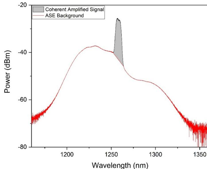
**Fig. 3.** Typical optical spectrum of an amplified pulse from the single pass configuration. The coherent amplified signal is indicated by the grey shaded area and sits on top of the ASE background shown in red.
