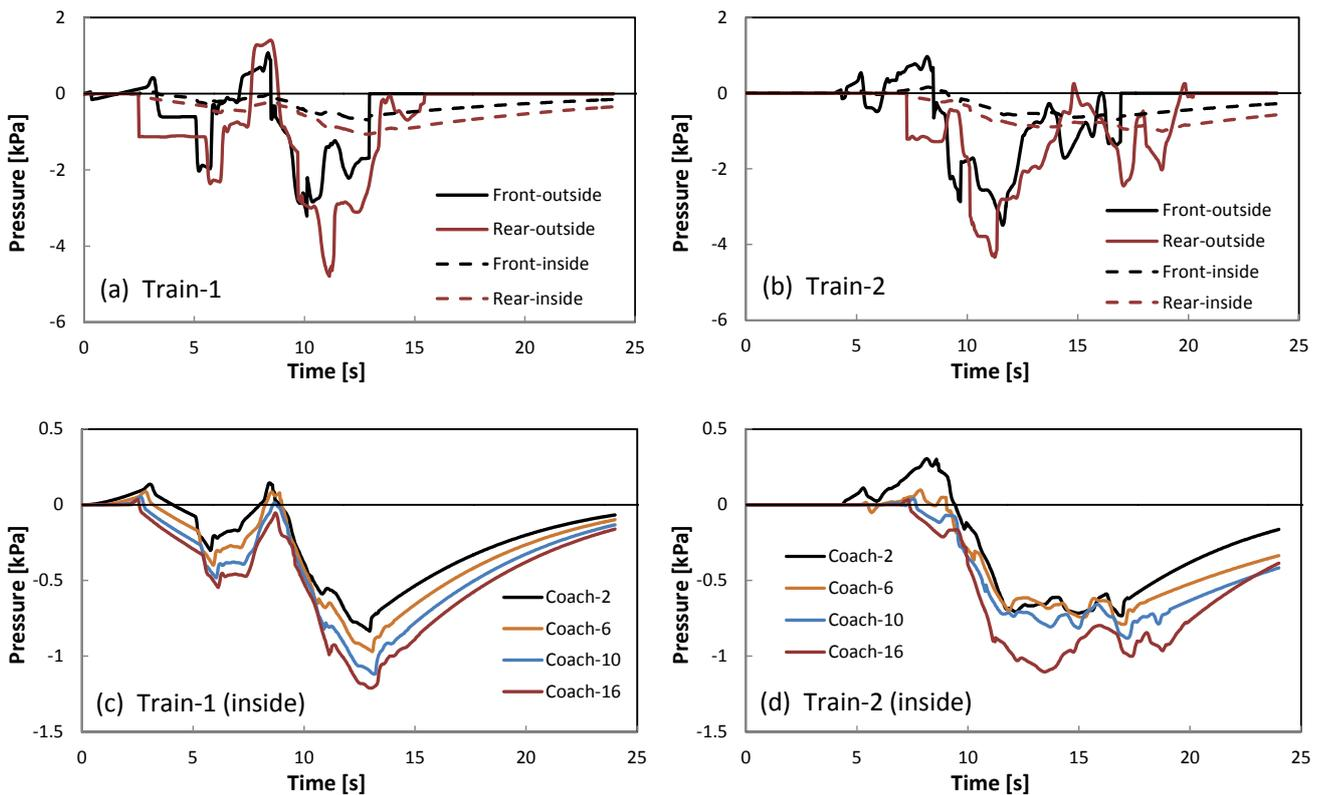
**Fig-1 Tendero Tunnel (horizontal), sealed trains at 300 km/h**
