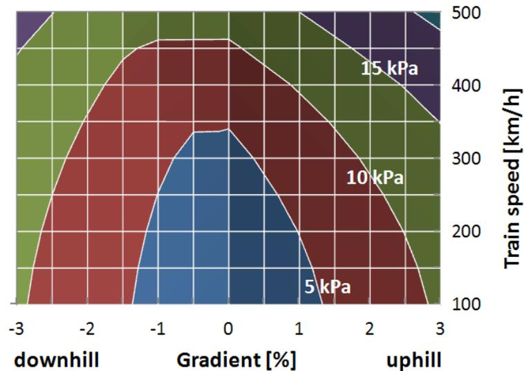
**Fig-4 Influence of elevation on maximum pressure change,  $L_t = 30\text{km}$ ,  $A_t = 50\text{m}^2$**
