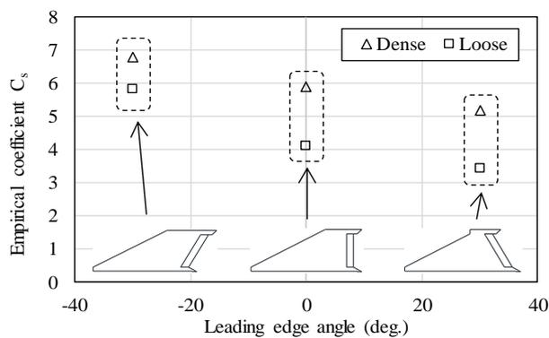
Fig. 7. Empirical coefficient  $C_s$  derived from the test against plough share leading edge angle.
