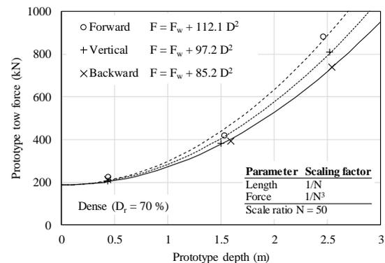
Fig. 6. Tow force against embedment depth for varying plough share leading edge inclination in dense sand ( $D_r = 70\%$ ).
