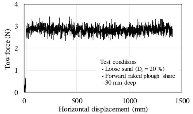
Fig. 4. Typical measured tow force (20% relative density, forward raked plough share and 30mm embedment depth)
