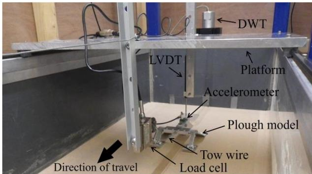
Fig. 3. Cable plough model before test commences.
