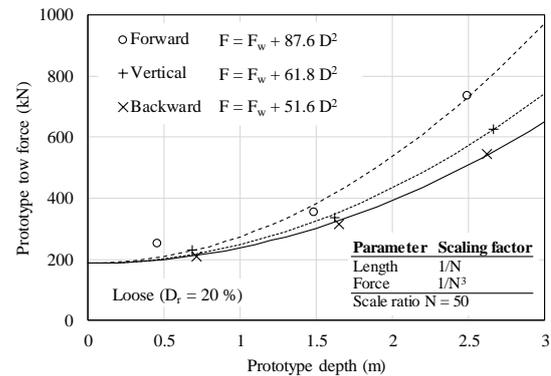
Fig. 5. Tow force against embedment depth for varying plough share leading edge inclination in loose sand ( $D_r = 20\%$ ).
