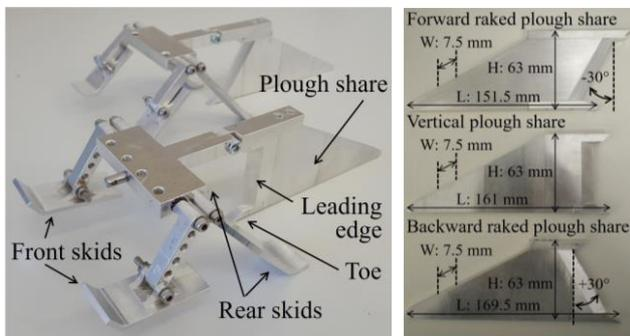
Fig. 1. 1/50<sup>th</sup> scale cable plough models and plough shares. models are displaced sufficiently to achieve the steady state (Robinson et al, 2016b). To provide actuation, a DC motor with a variable speed controller was used to move a platform mounted on low friction linear
