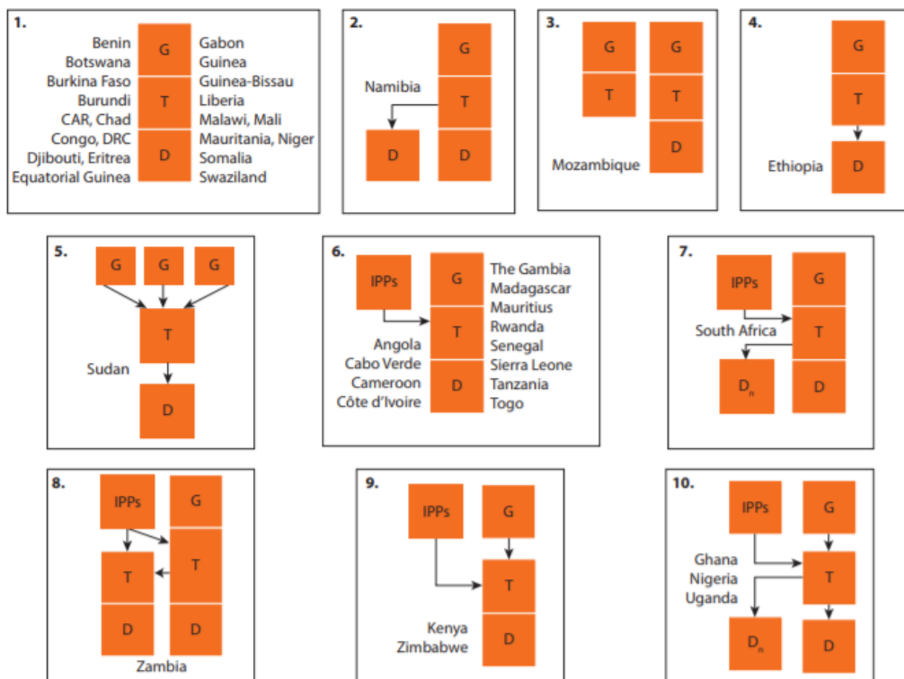
Figure 2.3 Electricity Structures in SSA
