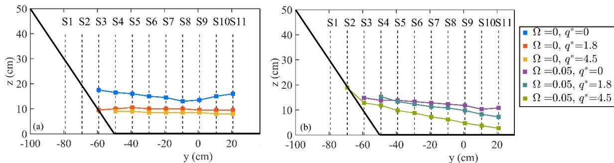
**Fig. 2.** Cross channel  $u=0$  cm/s velocity interface, for different  $q^*$  and angular velocity (a)  $\Omega=0$  rad/s and (b)  $\Omega=0.05$  rad/s.
