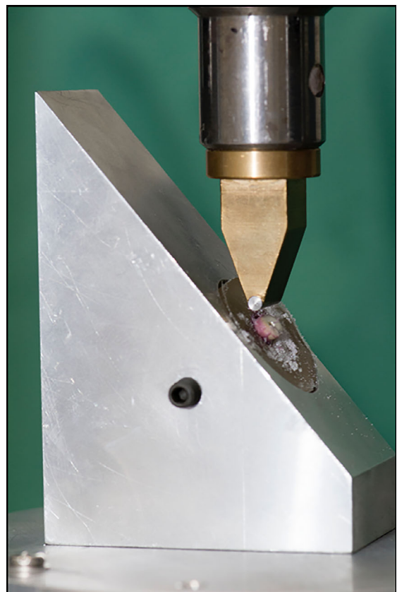
Figure 2 Sample mounting in the Instron® Testing Machine. Specimens fixed in a jig, with a chisel-shaped tip applied at 130° to the long axis of the tooth in a lingual-labial direction.
