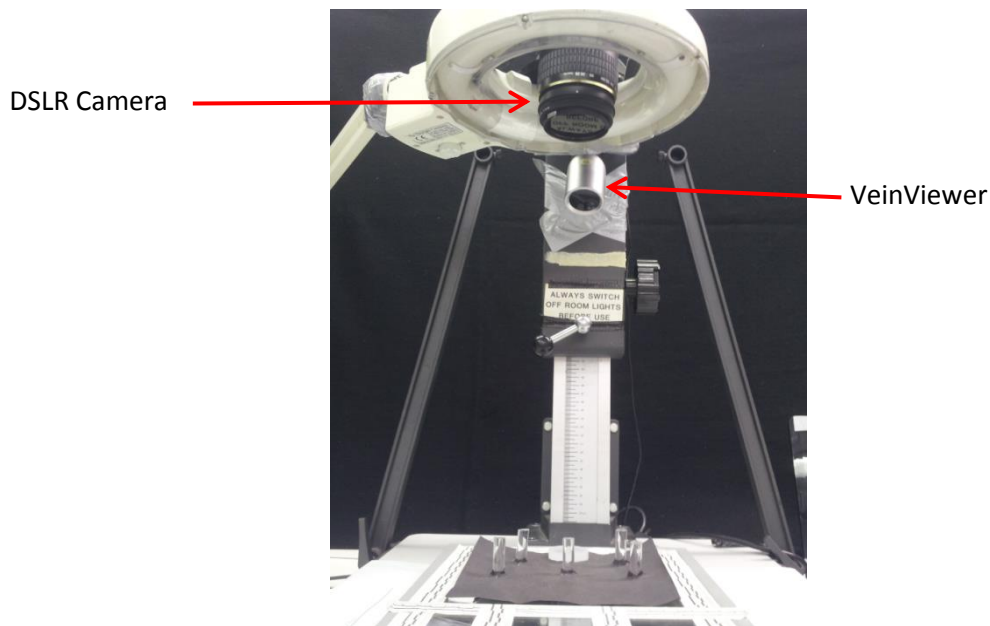
Figure 15. VeinViewer positioned below DSLR
