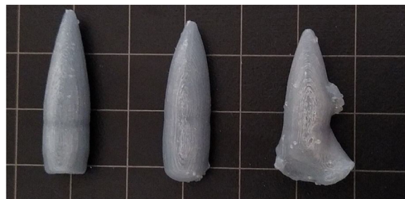
Fig. 5. 3D printed bullets (left) unfired bullets and (extreme right) fired and deformed bullets.
