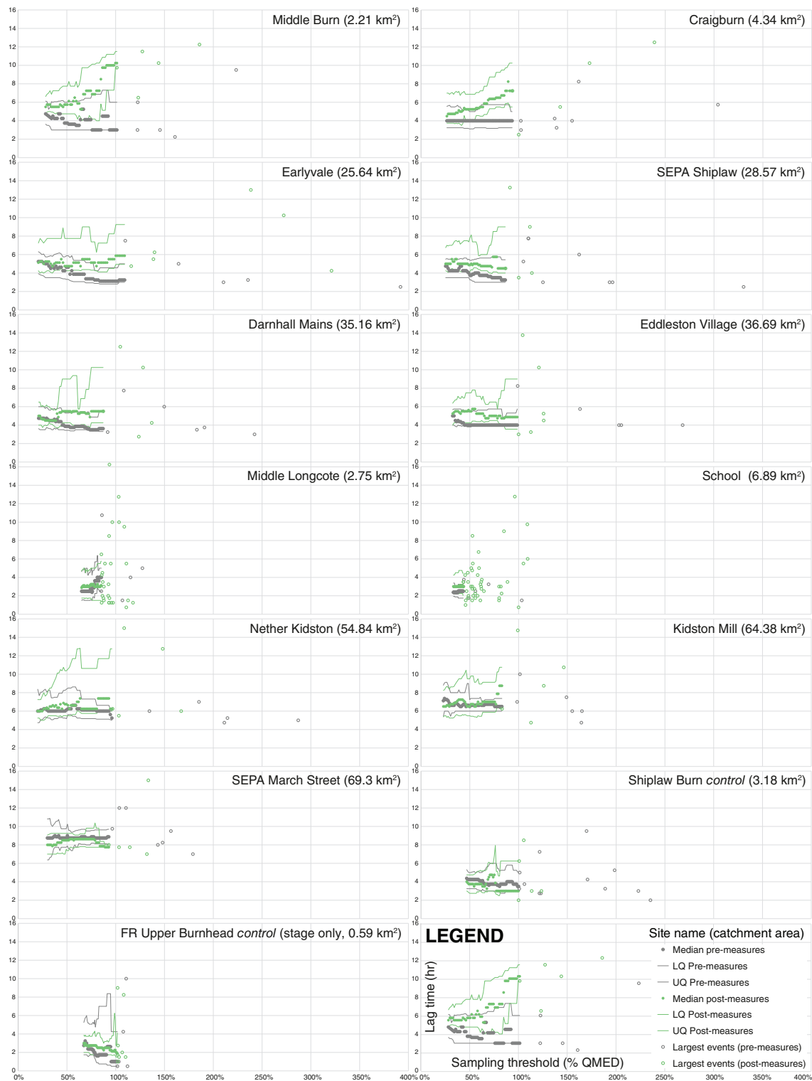
FIGURE 3 Median lag time for events in the baseline and experimental periods at different flow sampling thresholds (shown as a fraction of the median annual flood QMED). Median at each threshold in the different periods calculated as the median lag time for all events above the threshold, up to the point where the sample size in either period is <5. Open circles show lag for the largest individual events above this point. LQ/UQ: lower/upper quartiles. Sites are arranged upstream to downstream, with catchment area shown in each plot title. Sites are located on Figure 1. Details of natural flood management (NFM) interventions are in Table 1
