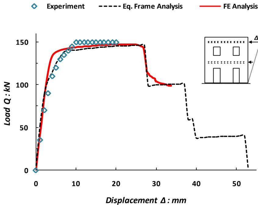
**Figure 3.** Calibration of nonlinear masonry material model with reference to pushover test results [Magenes et al., 1995] and comprehensive macroelement analysis using the Equivalent Frame Method [Galasco et al., 2004].
