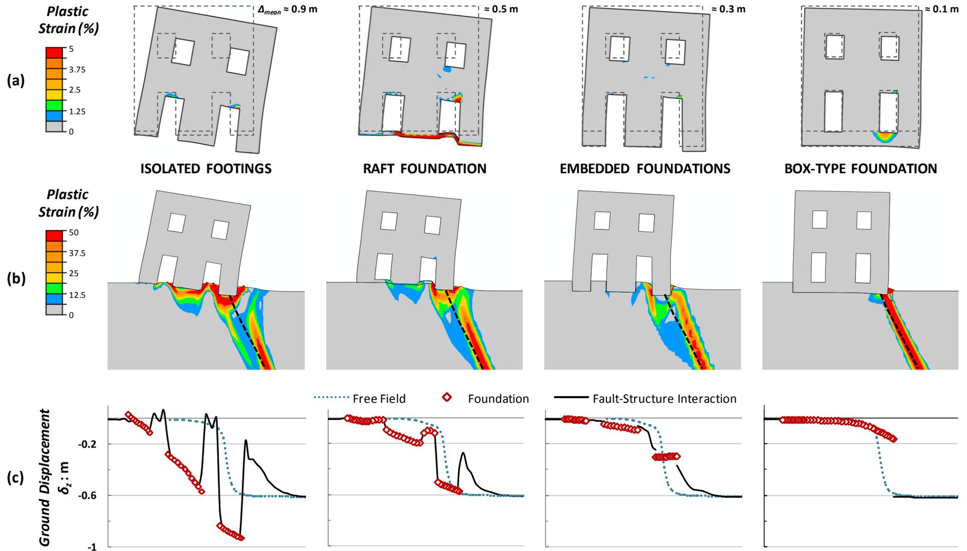
**Figure 7.** Effect of the foundation type for  $s/B = 0.88$  : (a) deformed masonry wall and (b) deformed soil–structure system with superimposed plastic strains indicating shear localization mechanisms for  $h = 0.6$  m; and (c) ground surface displacement profiles compared to free field response.
