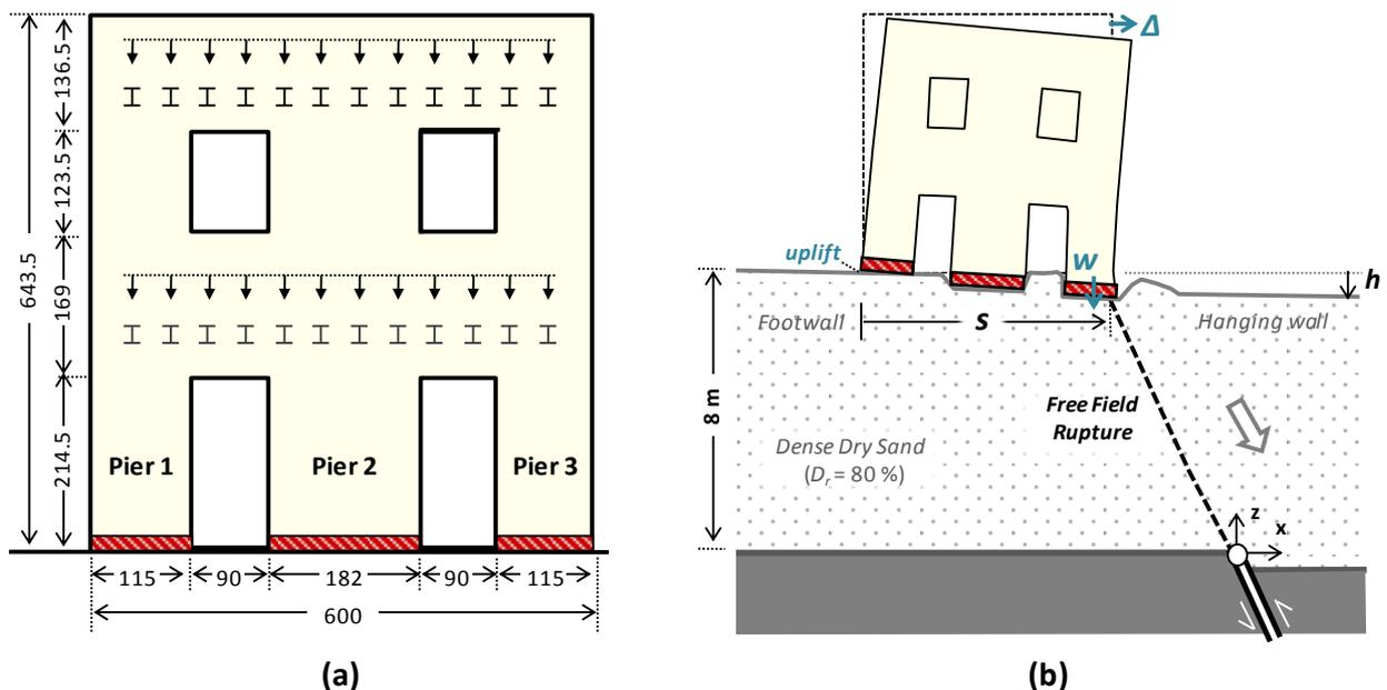
**Figure 1.** Definition of the problem: (a) Geometry of the masonry wall as adopted by Magenes et al., 1995 (with dimensions shown in centimetres); (b) Schematic of fault–soil–structure interaction mechanism and key parameters.
