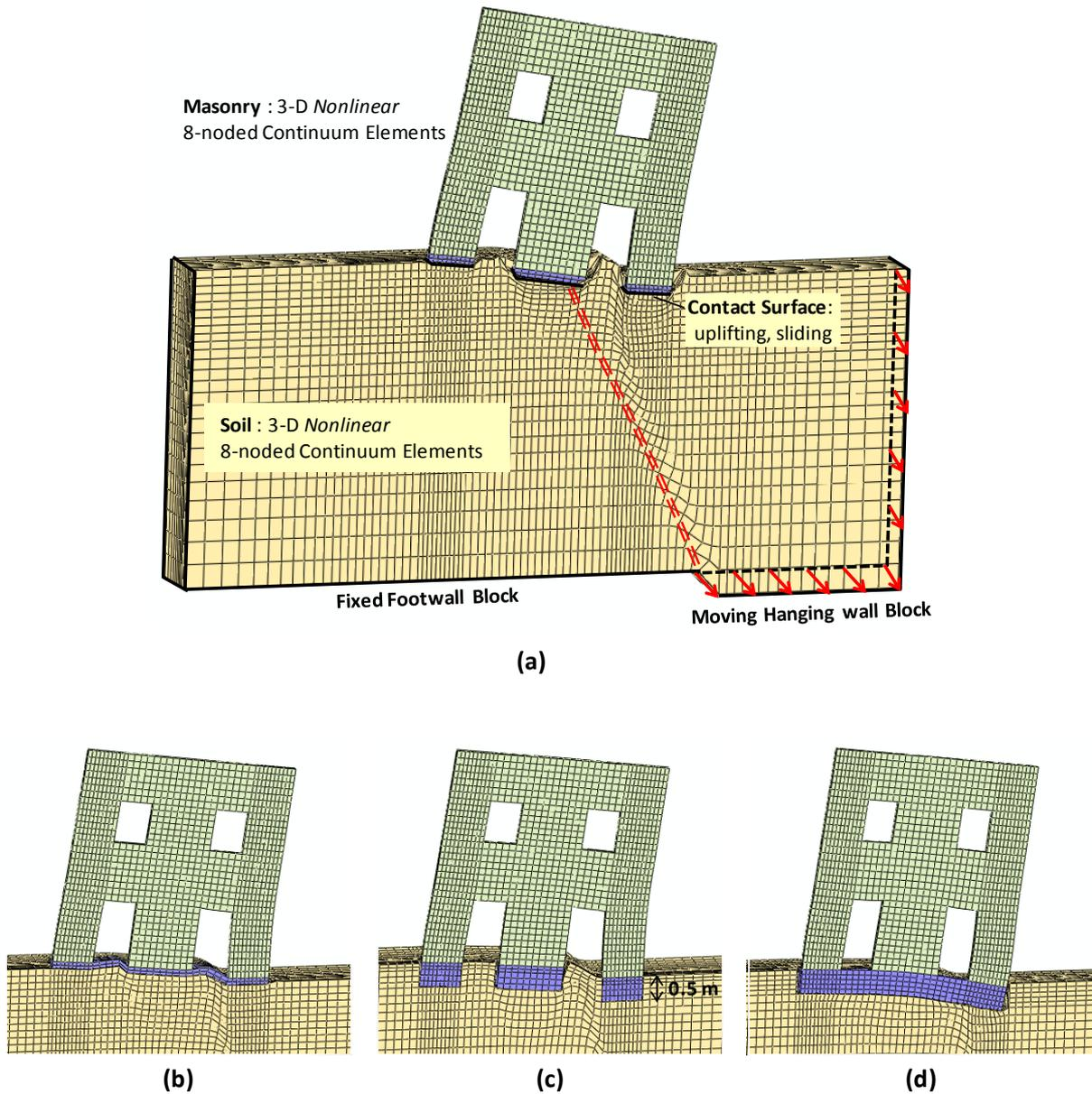
**Figure 2.** Numerical modelling details. (a) Deformed FE mesh for the benchmark case wherein the wall is supported on isolated footings; and the three foundation alternatives: (b) raft foundation; (c) embedded foundation; and (d) continuous box-type foundation.
