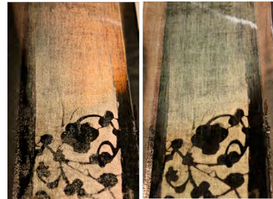
Figure 5. Shifts of surface colour as a result of the fibre optics on the liquid crystal printed linen.
