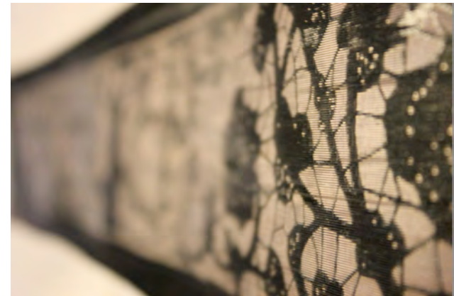
Figure 3. Screen printed white-scattering liquid crystal dyes
