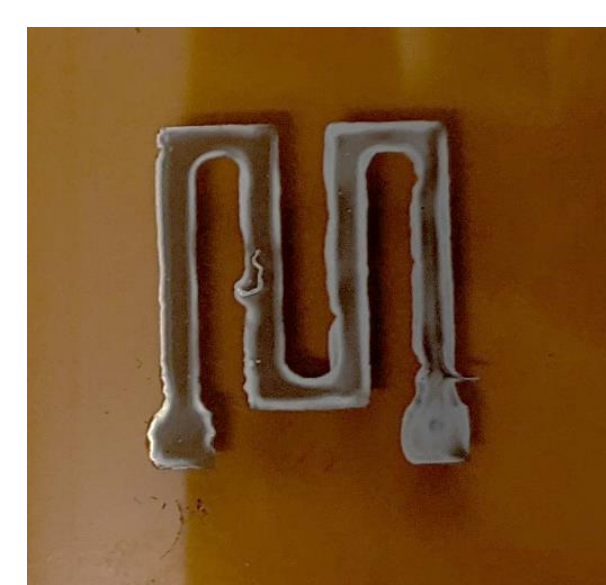
Sensor printed on Kapton
