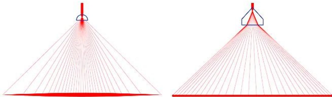
Figure 5-5. Highlighting the differences in the laser intensity distribution of a cylindrical lens (left) and a Powell lens (right) using ray traces. The Powell lens produces a much more even intensity distribution than the cylindrical lens.
