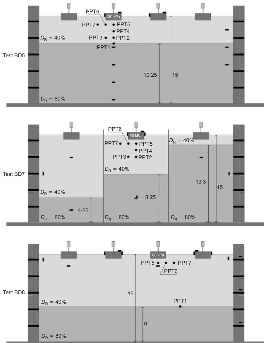
Fig. 1. Layout of centrifuge tests and instrument positions
