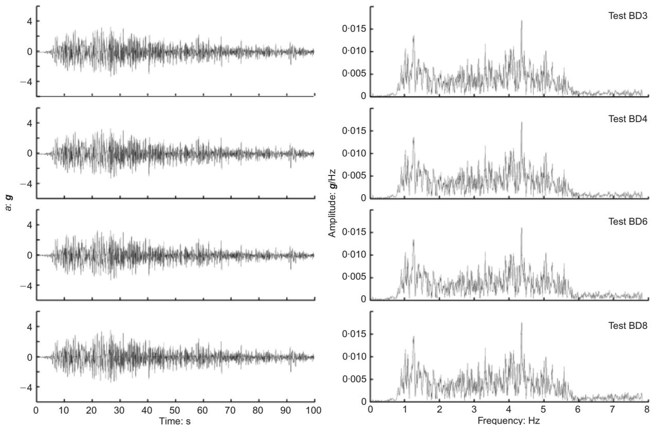
**Fig. 2. Acceleration record measured at the ‘Colegio Concepción’ station (San Pedro de la Paz) during 2010 Maule earthquake and earthquake motions reproduced in the centrifuge tests**
