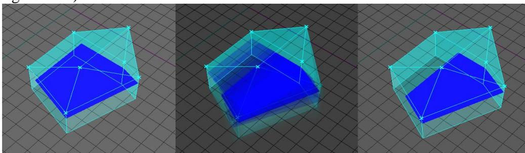
**Figure 10.** Defining the mezzanine floor relationship to the building form.
