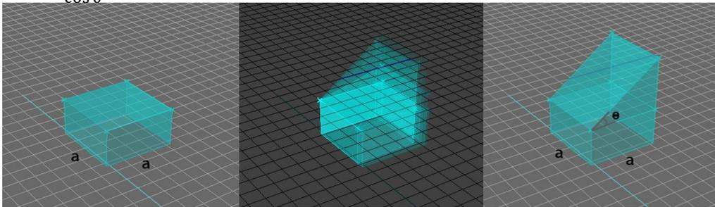
**Figure 7.** Relationship between side length of plan (a); angle of south roof ( $\theta$ ); area of south roof (S).
