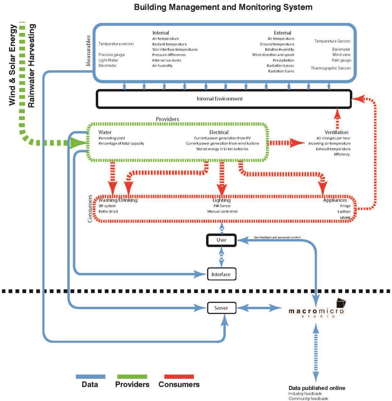
Figure 15. Schematic for proposed building management system
