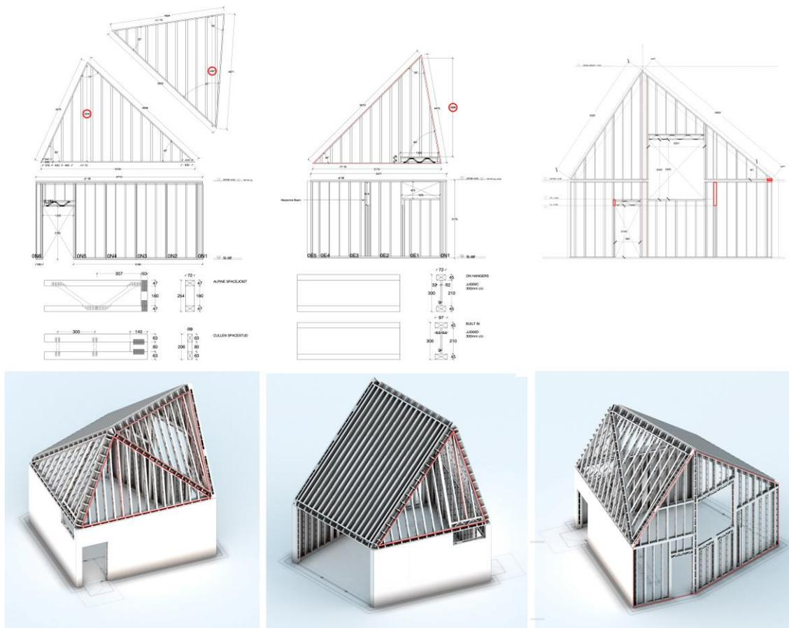
Figure 12. Timber frame design.
