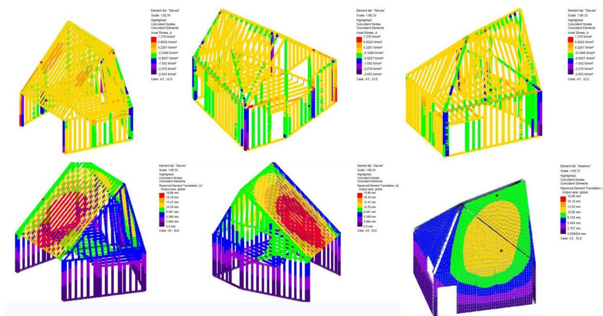
Figure 13. FEA analysis of building shell.
