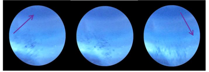
Fig. 5: (Purple arrows in each case represents direction of travel of MBs) Left: MBs approaching US focus. Middle: MBs reaching the US focus, beginning to change direction. Right: MBs completely changing direction due to acoustic radiation forces.
