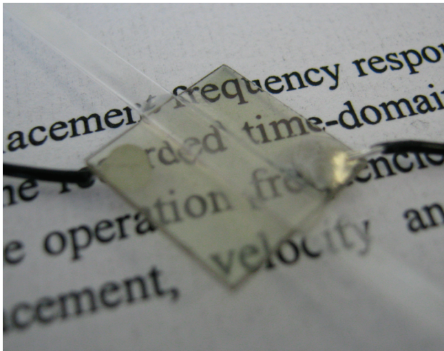
Fig. 1. A Y-36° cut lithium niobate plate coated with indium tin oxide and coupled to a glass capillary, showing its visible transparency.
