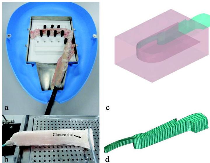
**Fig. 4 a** Operating platform - specimen was mounted with plastic bars. **b** Leakage pressure testing. The leakage pressure was recorded when the closed laceration first started to leak. **c** Geometry models of the clip and U-shaped-groove model. **d** Hexahedral mesh was generated to the clip.
