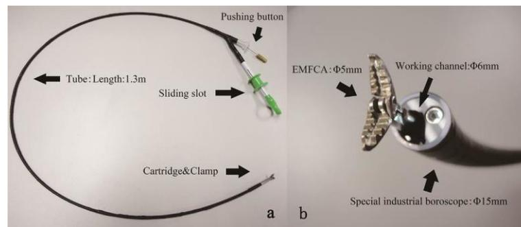
**Fig. 1** Prototype of EMFCA and modified boroscope.
