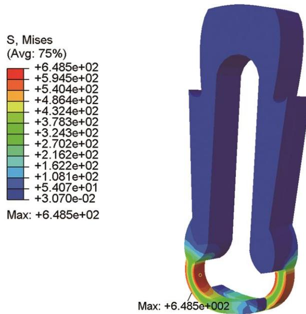
**Fig. 6** Mises stress contour of the clip in a symmetrical view. The maximum stress was 648.5 MPa and was located in thin arms.
